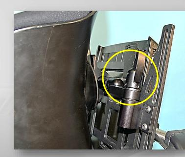
2. Release back support from frame and tighten back angle adjustment.
