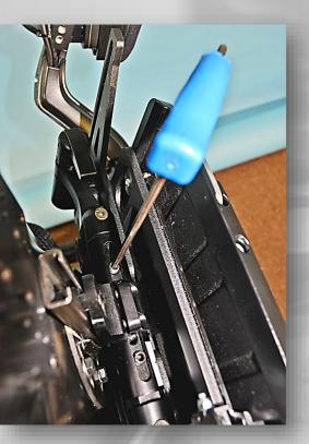
1. Tighten FlexLoc width and pivot screws.
